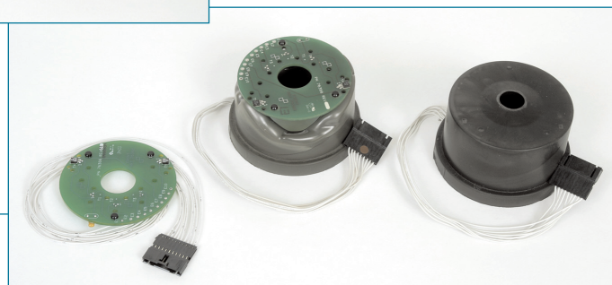
A 1/4" aluminum plate and a steel alloy strap are molded into a single part, as shown above. Encapsulation using RIM was chosen for two different applications on one product manufactured by Kendro Laboratory Products. Above (right), sophisticated electronics are encapsulated to protect against damage.
